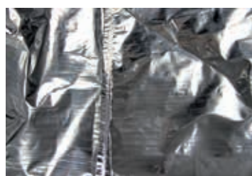
Radiation sterilised inliner With oxygen barrier and UV protection
